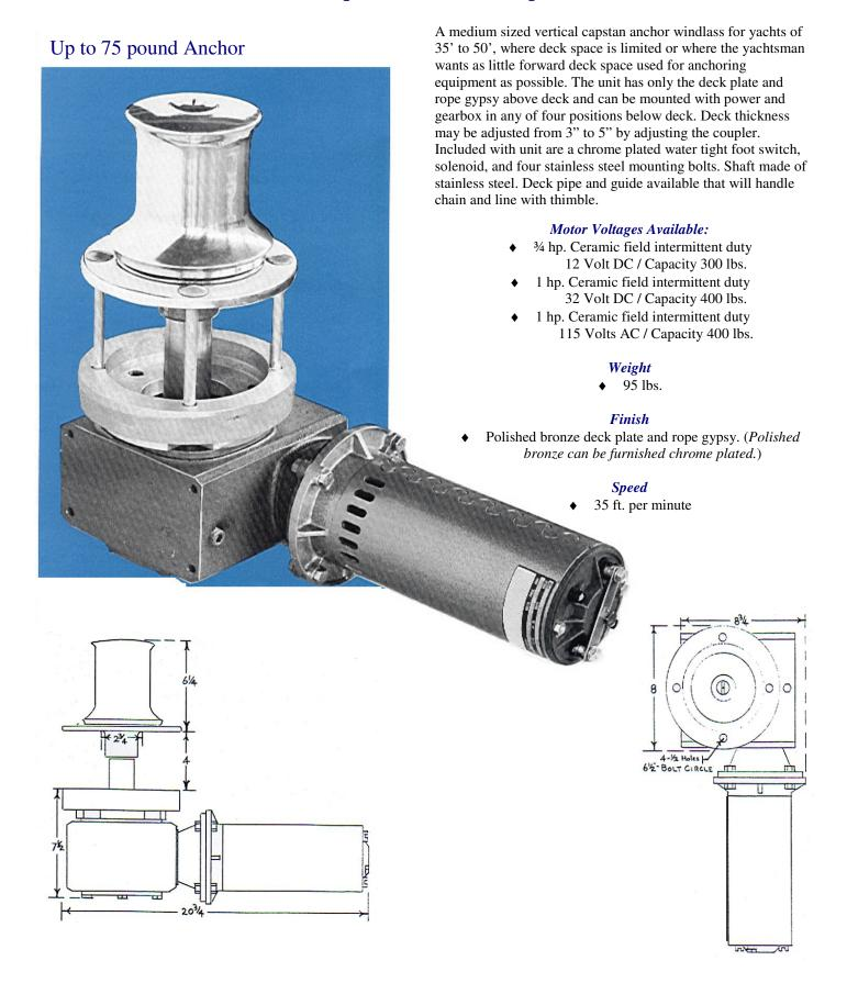
A medium size vertical anchor windlass for yachts of 35' to 50' where forward deck space is limited or where the yachtsman wants as little forward deck space used for anchoring equipment as possible. This unit is built with chain wildcat with cone clutch and rope gypsy. The rope gypsy may be used independently of the wildcat if desired. The power and gear box can be mounted in any of four positions below deck. Deck thickness may be varied from
