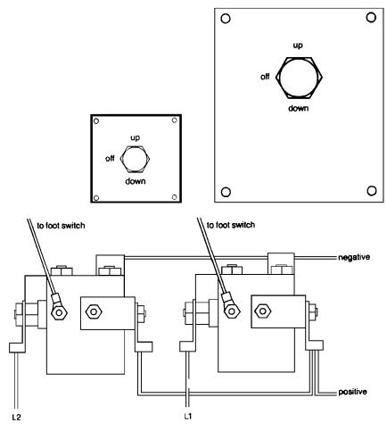
Power Up/Power Down Panel for 12 volt anchor windlass. Models 2, 3, 4, 5, 6, 9, 11, and 12.
